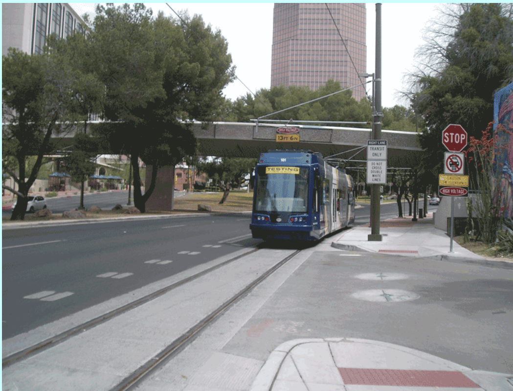
Figure 5 - Eastbound Single Track on Broadway, Part of Track Pair with Westbound Congress Street with County Government Complex in Background.
